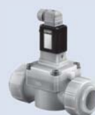
142 plastic solenoid valve, pvc, pvdf, pp, 1/2" - 2", 7 psi - 85 psi
