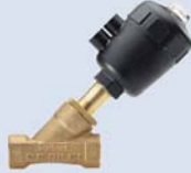
2000 pneumatic angle isolation valve for water/air/stream, 0 - 230psi, 3/8" - 2 1/2" 14F - 356F
